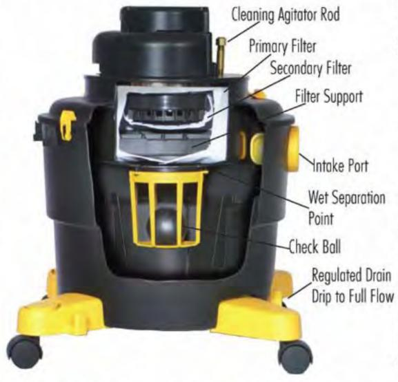
Dustless wet/Dry Vacuums come with fabric primary and secondary filters that are machine washable and designed for lifetime use.
